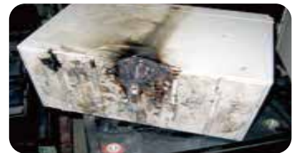
Leakage from battery bottom
